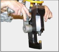
Both triggers must be depressed to close the unit and operate the peck cycle.
